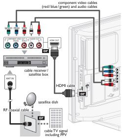
You can also connect this unit to the cable receiver or satellite box other than the HDMI or the component video output jacks because they might have different output jacks.
